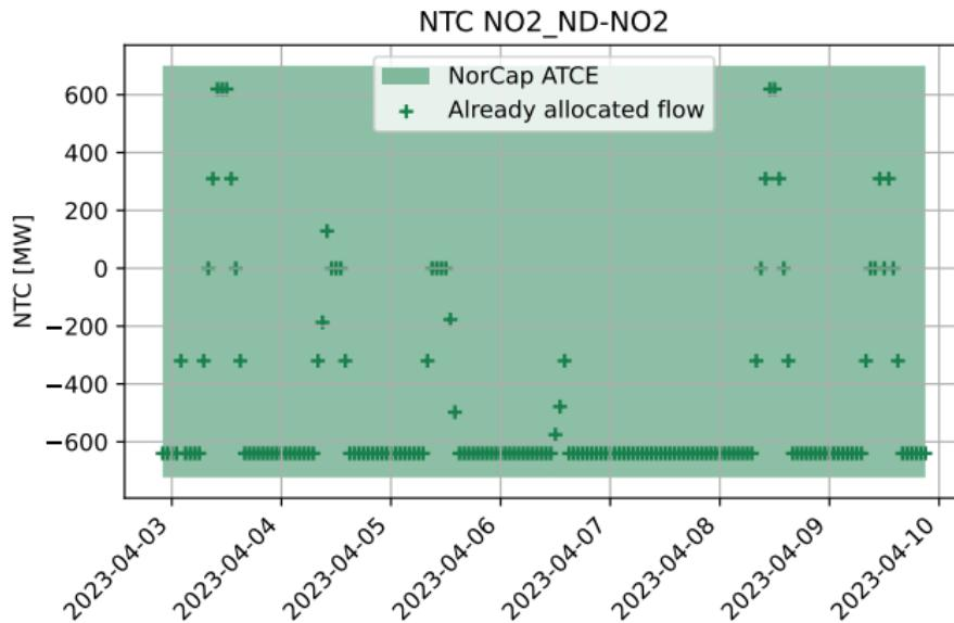
Note: NTC for NorNed includes 3.1% capacity reserved for losses. These will be subtracted in a future revision.
