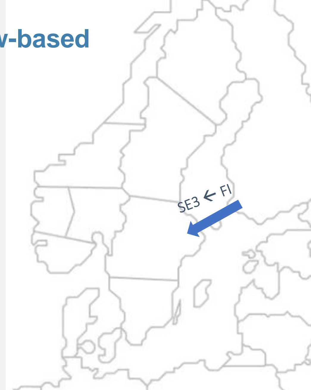
Figure: Fenno-skan interconnector is a combination of HVDC lines between FI and SE3.
